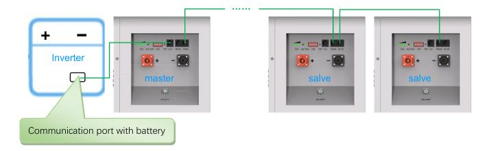
Note: Supports up to 16 sets of batteries in parallel
