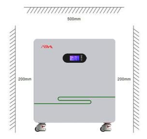
Note: This product is very heavy and must be installed on a flat and sturdy ground.
